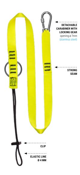
Tool lanyard – protection against dropping of tools, e.g. assembly wrenches. Strong seams, equipped with elastic line at one end, and stainless-steel detachable carabiner with opening of 7 mm at the other.
