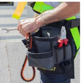
Hip tool belt fastened using connecting and adjusting buckle. Provides optimum arrangement and handling of tools which in turn improves working comfort.
