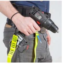
Tool lanyard – protection against dropping of tools, e.g. assembly wrenches. Strong seams, equipped with elastic line at one end.
