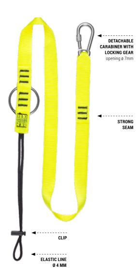
Tool lanyard – protection against dropping of tools, e.g. assembly wrenches. Strong seams, equipped with elastic line at one end, and steel detachable carabiner with opening of 7 mm at the other.
